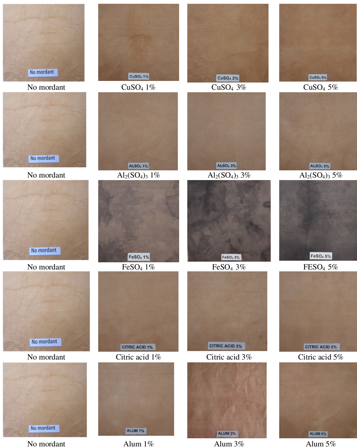
Fig. 2. Colours of silk fabric treated with different mordants and dyed with cashew nut peel.
